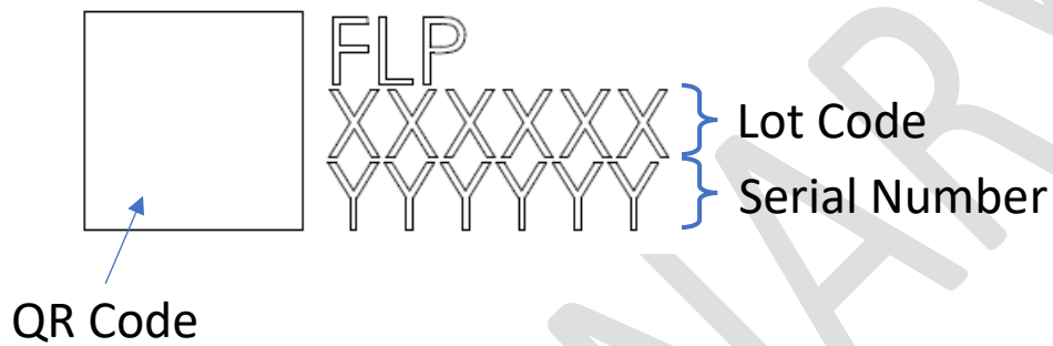
Figure 6. Details of Azumo product serial code.
