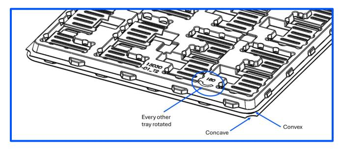
Figure 17. Required rotation of every other tray to avoid damage to products.
