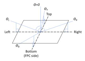
Figure 2. Definition of viewing angles relative to LCD display.
