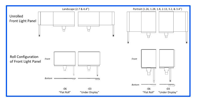
Figure 8. -06 and -03 roll configurations of the Azumo LCD 2.0 FLP
