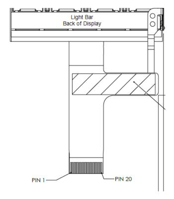
Figure 1. Detail of LCD FPC.
