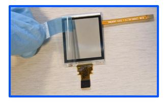
Figure 12. Removal of protective liner using speedy tab.
