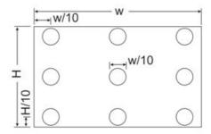
Figure 4. Testing regions for brightness and uniformity.
