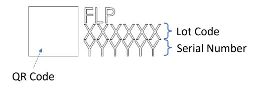
Figure 6. Details of Azumo product serial code.
