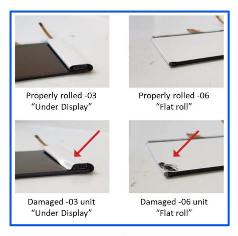
Figure 14. Examples of damage to FLP roll.
