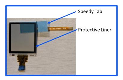
Figure 11. Identification of protective line and speedy tab.
