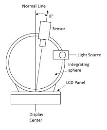
Figure 3. CM700d - Diagram of measurement equipment for contrast ratio.
